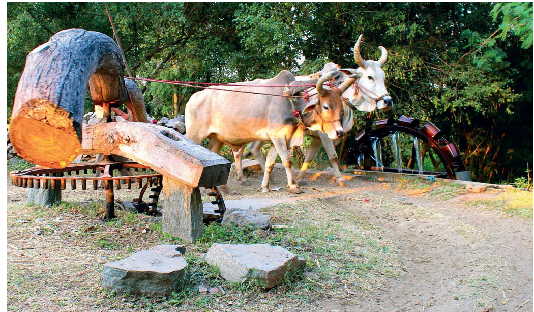
Persian wheel used for lifting water from the well
