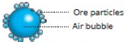
Enlarged view of air bubble showing the ore particles attached to it.
