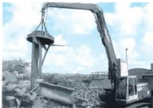
a. used in scrap yard to lift ferrous metals
