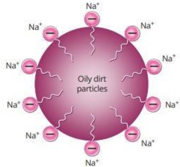
A spherical micelle formed by soap in water
