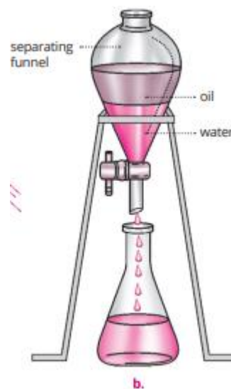
b. Separation of two layers forms the oil layer at the top and water layer at the bottom
