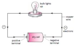
The flow of electrons in a wire is electric current.
