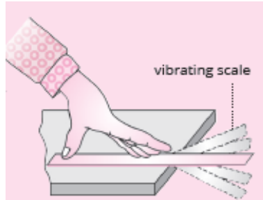
A vibrating scale produces sound
