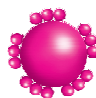
Enlarged view of an air bubble showing the ore particles attached to it.
