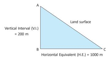
In this right-angled triangle, CA is the distance to be travelled to gain the height AB (200 metres). AB is the vertical interval (V.I.) which can be easily found from the contours. BC is the horizontal equivalent (H.E.), which can be easily measured from the contour map. The ratio between V.I. and H.E. gives the measure of the steepness and is called the **gradient**.
